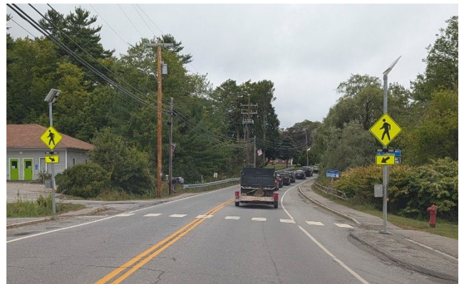
Exhibit 12. Rectangular Rapid Flashing Beacon
